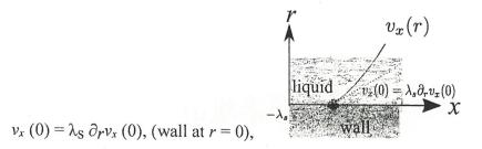
where  $\lambda_S$  is the slip length or Navier length defined as the distance behind the boundary where the tangent of the velocity field intersects the x axis. Note that for  $\lambda_S = 0$  we recover the usual no-slip boundary condition.
