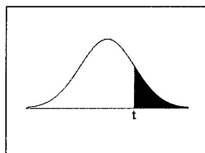
The shaded area is equal to  $\alpha$  for  $t = t_\alpha$ .
