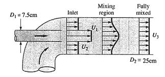
(25%) Flow through the converging nozzle can be approximated by the one-dimensional velocity distribution
