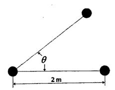
2. (20%) A 2-kg disk rests on a smooth horizontal plane and is attached to an elastic cord that has a stiffness of  $k_c = 20 \ N \ / m$  and the unstretched cord length is 0.5 m. Initially unstretched; if the disk is given a velocity  $v = 1.5m \ / s$  perpendicular to the cord, please use the conservation of angular momentum and conservation of energy to find the speed of the disk at the instant the cord is stretched 0.2 m. O is the center of rotation.
