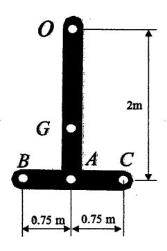
5. (20%) The uniform 50-kg bar is held in the equilibrium position by cord AC and BD. Determine the tension in BD and the angular acceleration of the bar immediately after AC is cut.
