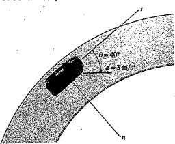
5. Determine the banking angle heta for the race track so that the wheels of the racing cars when it will not have to depend upon friction to prevent ant car from sliding up or down the track. Assume the cars have negligible size, amass m, and travel around the curve of radius  $\rho$  with a speed  $\nu$ . [20]
