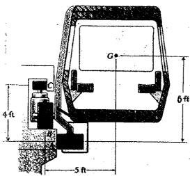
3. The vehicle has a weight of 2600 lb and the center of gravity at G. Determine the horizontal force P that must be applied to overcome the rolling resistance of the wheels. The coefficient of rolling resistance is 0.5 in. The tires have a diameter of 2.75 ft. [20]
