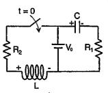
14. What is the potential difference  $V_C$  on the capacitor and the current  $I_L$  on the inductor at  $t = 0^+$ , instantaneously after the circuit is closed?
