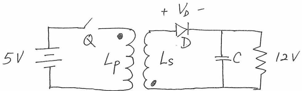
$f_{\text{switch}} = 100 \text{ KHz}$ ,  $L_p = 100 \mu\text{H}$ ,  $L_s = 200 \mu\text{H}$ ,  $P_o$  (output power) = 72 Watts. Assume ideal components
