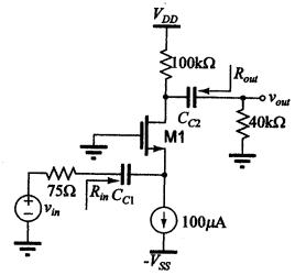
2. (15%) The following circuit is an active inductor; please derive the inductance  $L_{eq}$  with respect to frequency.
