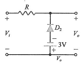
(b) Please plot the transfer curve ( $V_i$  is the x-axis and  $V_o$  is the y-axis) for the circuit on the left. For  $D_2$ , forward voltage  $V_F = 0.7 \text{ V } (6\%)$
